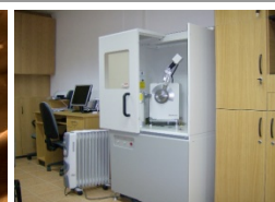
Vitreous \text{TeO}_2\text{-PbO-Ag}_2\text{O-Eu}_2\text{O}_3 SHIMADZU 6000 diffractometer
